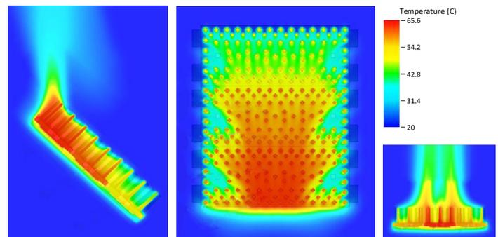
Heat sink to ambient temperature rise  $T_{hs-amb}$  (°C)
